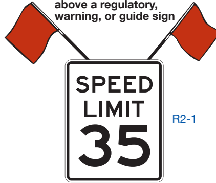
Figure 2A-1. Examples of Enhanced Conspicuity for Signs
